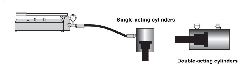
**Single-acting cylinders:** Position the cylinder so that the piston rod is pointed down and so that the cylinder is lower than the pump. The piston rod need fully extend and retract for two or three times.
