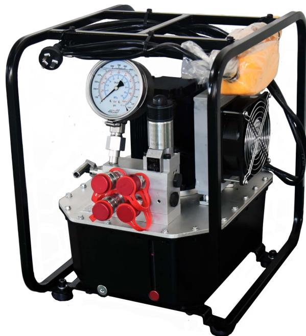
It is operating manual of KLW4020Z4 series Electrical Torque Wrench Pump, please read carefully follow instructions, warnings and cautions before using the tools.
